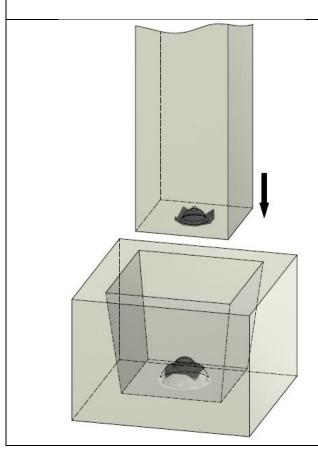
After the mortar is hardened around the foundation connector, the column can be installed.
