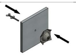
The column connector is fixed to formwork using a threaded bar and two wing nuts.
