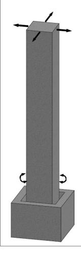
The connectors permit the column to pivot and maintain a fixed contact point.
