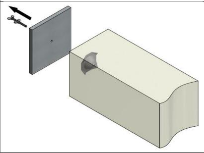
At the end, after the concrete has hardened, the threaded bar is unscrewed, and the formwork can be removed.
