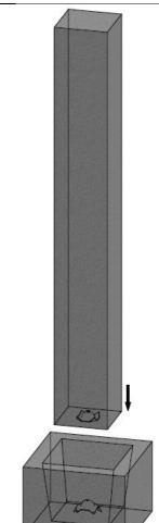
The foundation blocks aligned and installed on site, with the foundation connector embedded can now be used.
